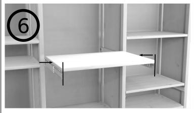
Bring in the shelf and make sure it is aligned with the front edges of the sliders and symmetrical on left and right sides.
