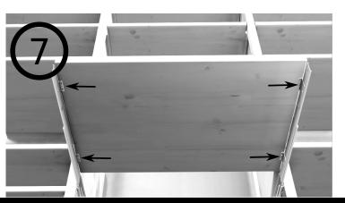
Secure the shelf a with screws to complete the installation.
