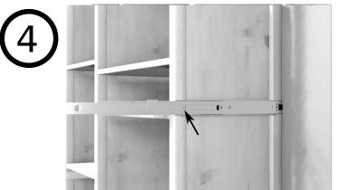
Open the slider **b** further to reveal the front hole and fix with a screw.
