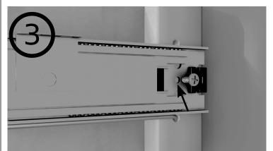
Open the slider **b** to reveal the screw hole and fix with a screw **c** to the back of the upright.
